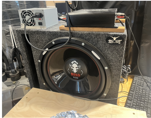
Figure 7: Image of large speaker used for excitation.
