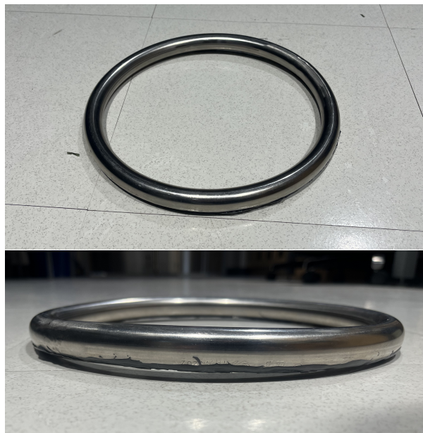
Figure 4: Top and side views of the original rung used to border the membrane.
