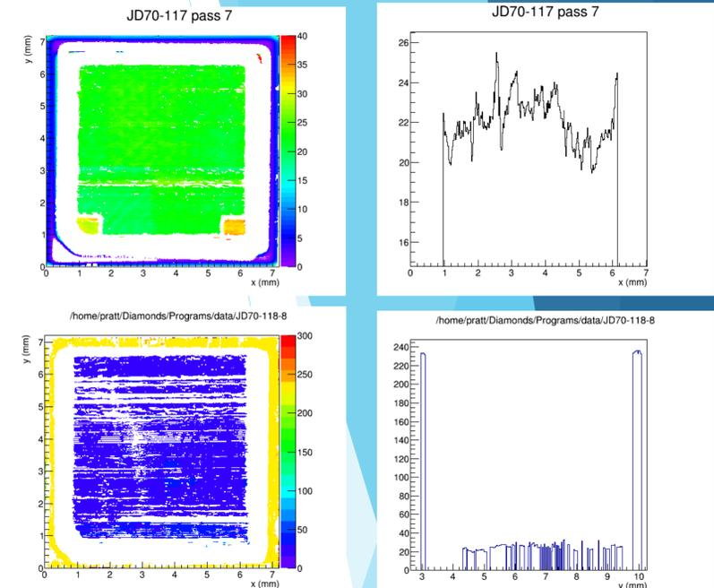
Figure: Zygo image of JD70-117 cut to 23 microns. The plot on the right is a cross section through  $y = 3.5$ mm
