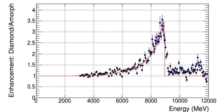
Figure: Initial data taken during Hall D Spring 2016 run using diamond JD70-118. The results show the photon beam enhancement of the diamond radiator when compared to an amorphous radiator.
