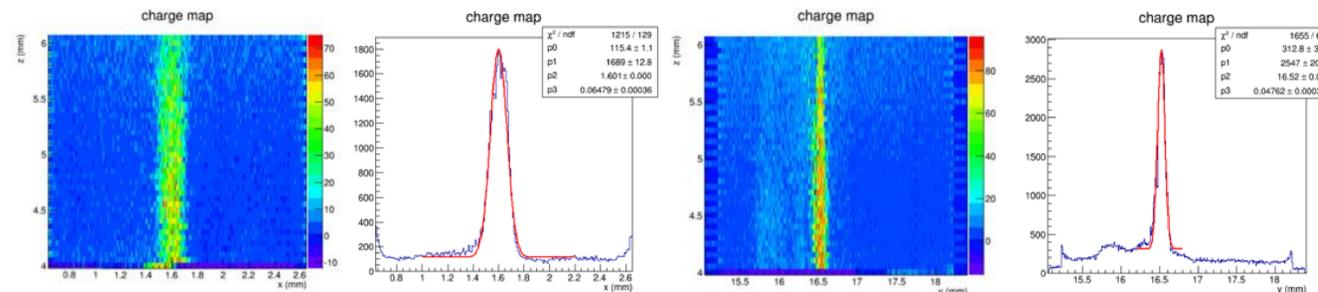
Figure: Color maps of the two orthogonal scans of the beam focal region, where the color represents the charge per pulse seen on the wire in arbitrary units. Projections of the wire charge maps onto the transverse axis with Gaussian fits to the central peak over a flat background.
