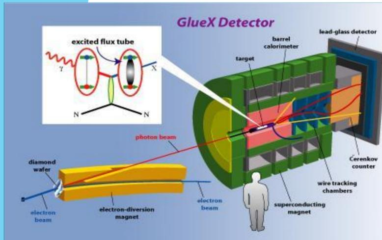
The GlueX experiment at the Thomas Jefferson National Lab in Newport News Virginia uses a polarized beam of 9GeV photons incident on a liquid hydrogen target to explore the excitations of gluonic bonds between quarks. 9GeV photons are generated by a 12GeV electron beam passing through a 20 $\mu$ m thick diamond wafer and undergoes coherent bremsstrahlung.
