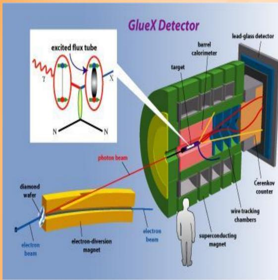
The GlueX experiment at the Thomas Jefferson National Lab in Newport News Virginia is a photonuclear experiment design to explore the excited gluonic bonds between quarks. A beam of polarized photons will be set incident on a 30cm liquid hydrogen target. To create a well collimated polarized photon beam, coherent bremsstrahlung radiation was chosen.
