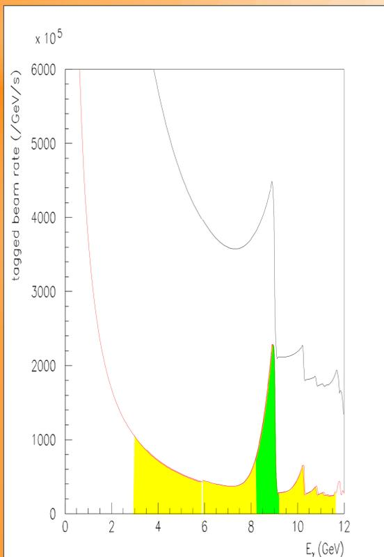
Bremsstrahlung produces electromagnetic radiation when a charged particle is deflected by another particle. In the GlueX experiment, a 12GeV electron will decelerate when it passes through a diamond radiator producing photons with about 9GeV. In order to create the sharp peak in the otherwise smeared bremsstrahlung radiation energy spectrum, the resulting photon beam will be collimated, also known as coherent bremsstrahlung.
