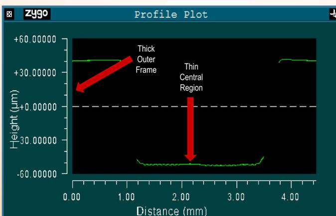
The plot below shows a cross section of sample S150 taken with a Zygo white light profilometer. After 100 $\mu$ m was removed from the central region, the interior surface remained exceptionally flat and the vertical walls steep; both of which are crucial requirements for the GlueX experiment.
