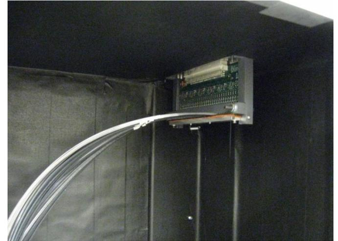
The fibers are bundled as 5 rows and 6 columns where each column corresponds to a different energy and the rows are used for calibrating the electron plane.
