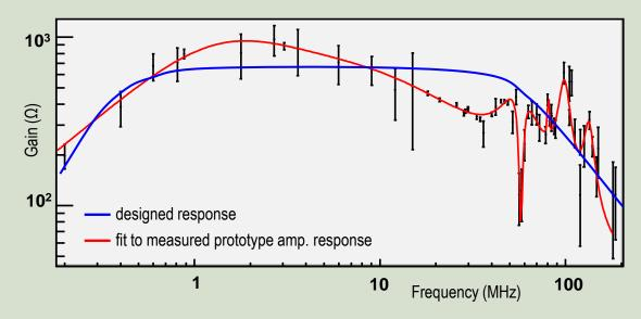
The frequency response of the prototype was measured using the FFT of an oscilloscope waveform.
