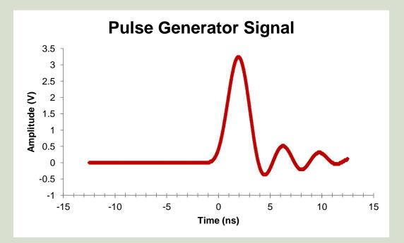
The signal from the pulse generator has a FWHM of 2.5ns and peak amplitude of 3.25V. The ringing is an artifact of the oscilloscope bandwidth of 200MHz. The laser diode has a threshold voltage of 2.7V, so it is only on for less than a nanosecond.
