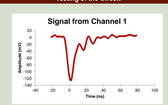
Above is the signal from the first individual channel on the prototype amplifier. A new design of the amplifier has been developed to eliminate the ringing seen in the signal.
