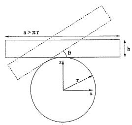
(a) Show that the coordinates of the center of gravity of the block are given by the following relations in a coordinate system with the origin at the center of the cylinder.
