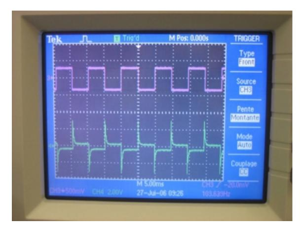
(Fig. 2. The display panel of the oscilloscope showing the electrical potential before and after the Operational Amplifier circuit)
