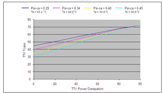
Figure 8-4. Example: Required  $\Psi_{CA}$  for Various  $T_{AMBIENT}$  Conditions
