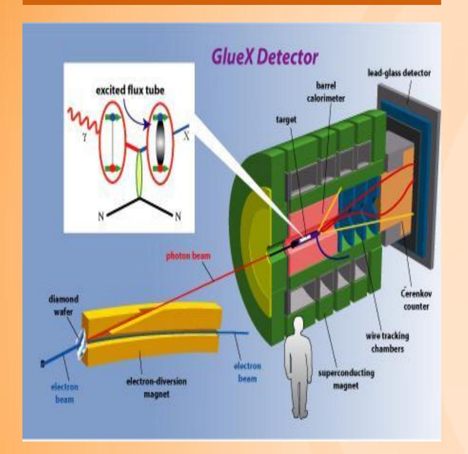
The GlueX experiment at the Thomas Jefferson National Lab in Newport News Virginia is a photonuclear experiment design to explore the excited gluonic bonds between quarks. A beam of polarized photons will be set incident on a 30cm liquid hydrogen target. To create a well collimated polarized photon beam, coherent bremsstrahlung radiation was chosen.
