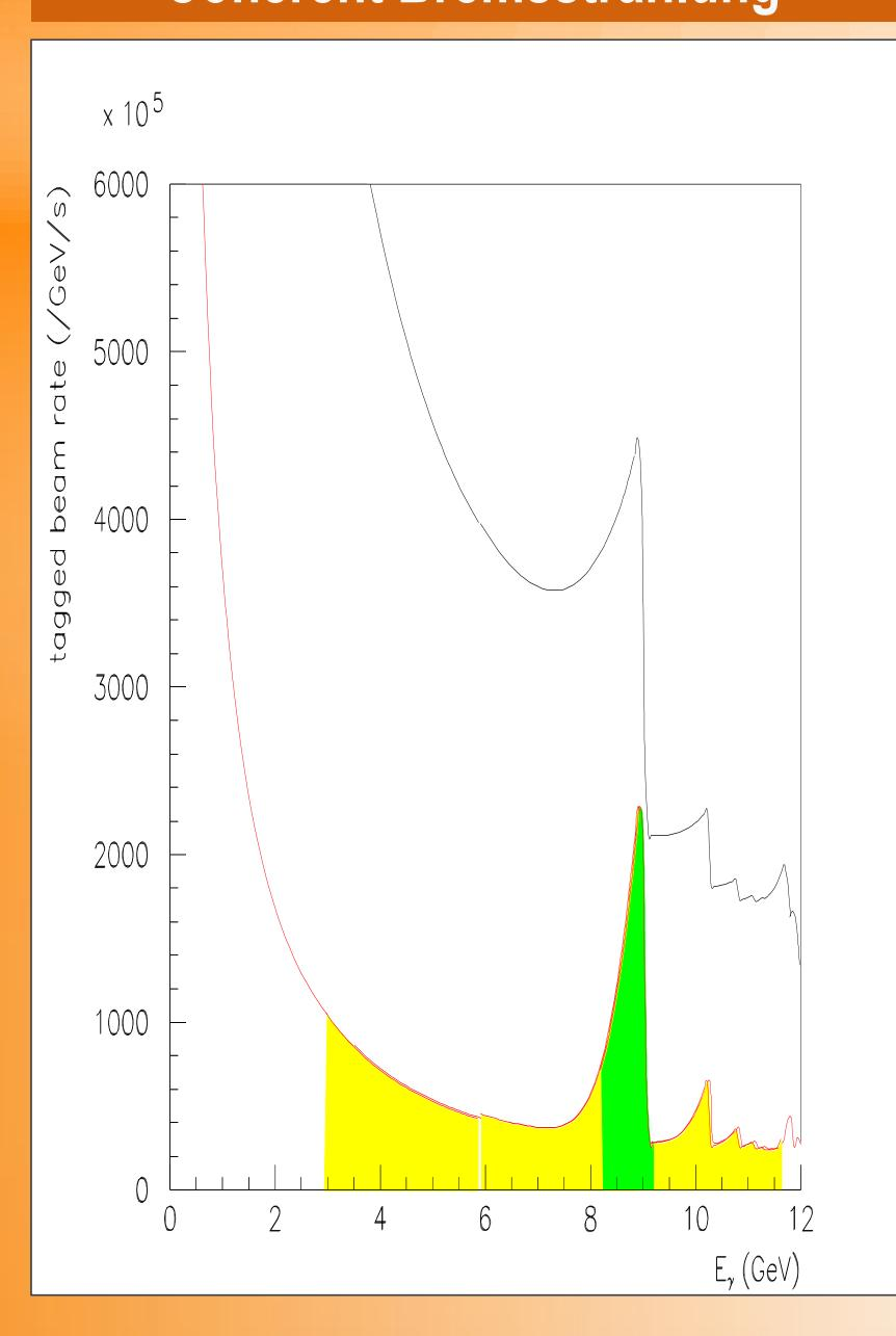
Bremsstrahlung produces electromagnetic radiation when a charged particle is deflected by another particle. In the GlueX experiment, a 12GeV electron will decelerate when it passes through a diamond radiator producing photons with about 9GeV. In order to create the sharp peak in the otherwise smeared bremsstrahlung radiation energy spectrum, the resulting photon beam will be collimated, also known as coherent bremsstrahlung.
