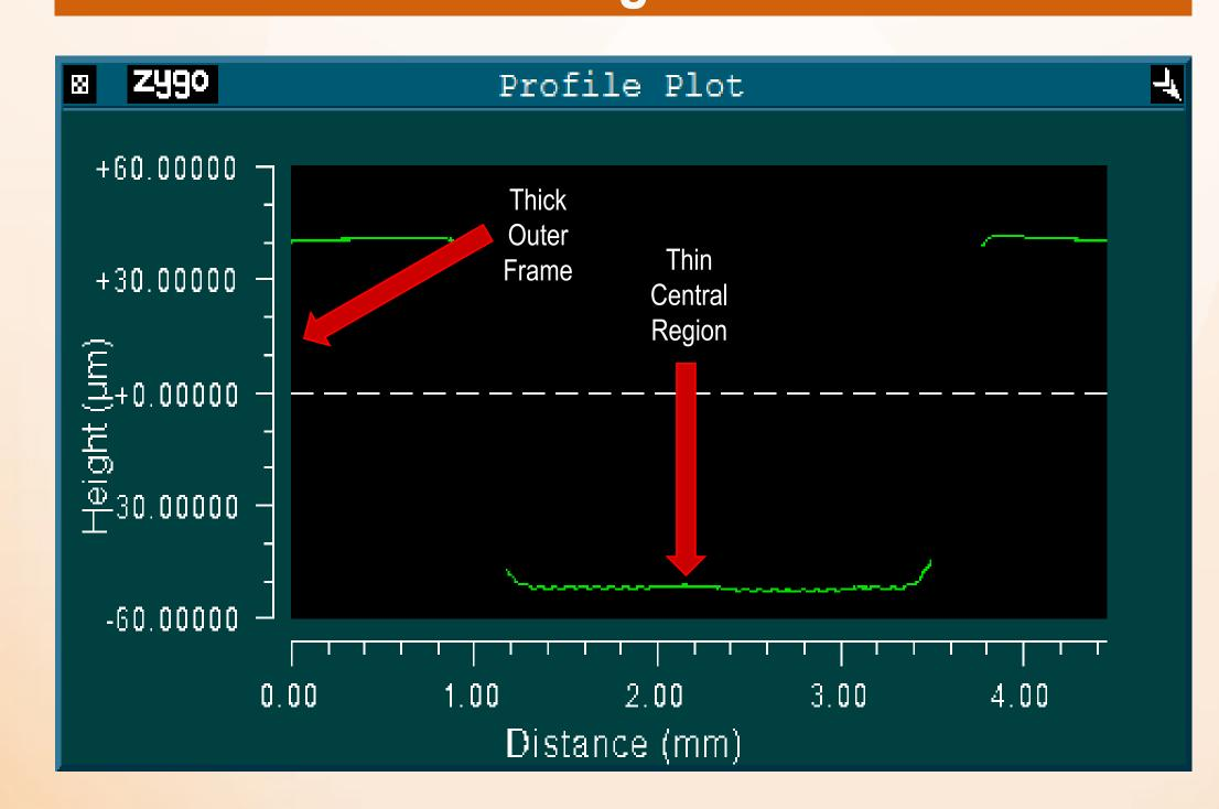
The plot below shows a cross section of sample S150 taken with a Zygo white light profilimeter. After 100µm was removed from the central region, the interior surface remained exceptionally flat and the vertical walls steep; both of which are crucial requirements for the GlueX experiment.
