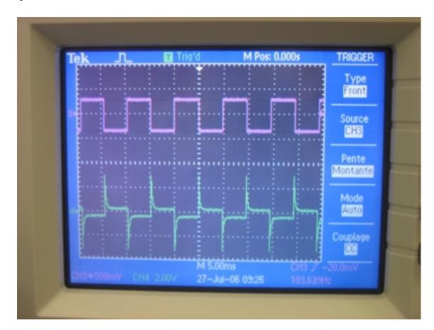
(Fig. 2. The display panel of the oscilloscope showing the electrical potential before and after the Operational Amplifier circuit)
