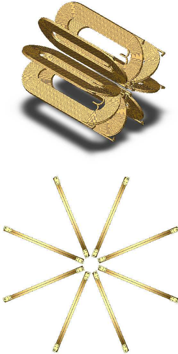
Figure 72: The radial arrangement of the Q_{Weak}^p Toroidal Magnet coils. The drawing is done by BATES engineer Stan Sobczynski.
