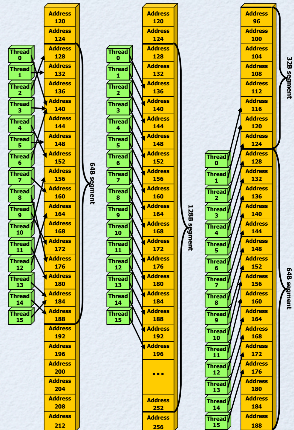
Left: random float memory access within a 64B segment, resulting in one memory transaction. Center: misaligned float memory access, resulting in one transaction. Right: misaligned float memory access, resulting in two transactions.
