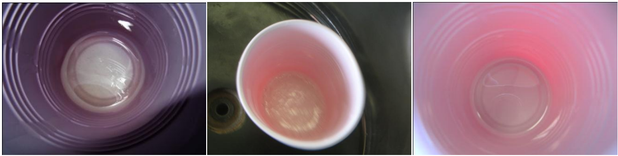
Figure 24: Stages of removing entrained air from the glue.
