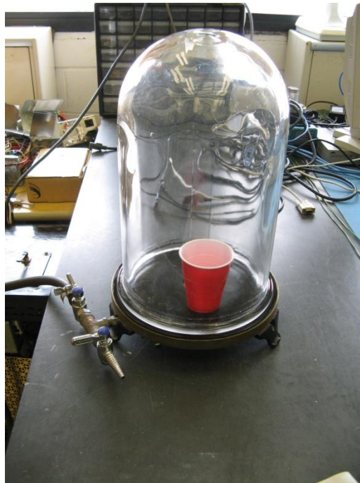
Figure 23: Vacuum chamber set-up. The red cup contains a sample of mixed epoxy.
