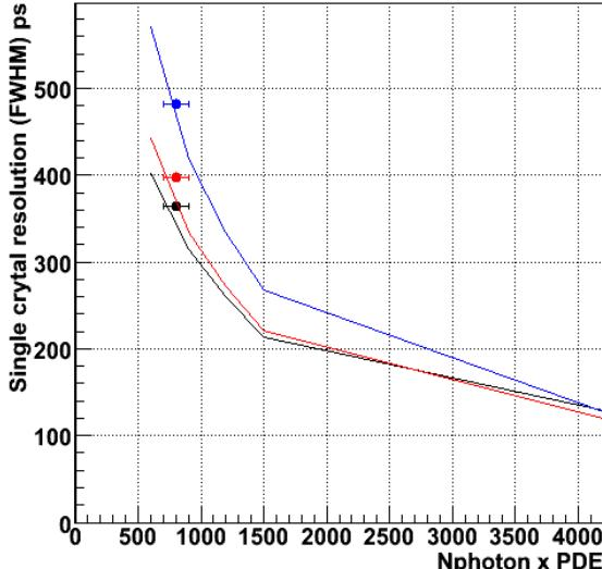
. Fig. 7. Comparison of the timing resolution obtained in data (points) and simulations (lines). The colors correspond to 3 different thresholds. 40 mV ( $>6\text{PE}$ ): blue, 18 mV (3 PE): red, 12 mV (2 PE): black.
