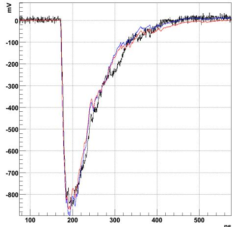
Fig. 5. Comparison of waveform for data (black) and simulations (blue and red). Two different pulse shape were used for the simulated waveforms: SPICE for the blue, empirical for the red.
