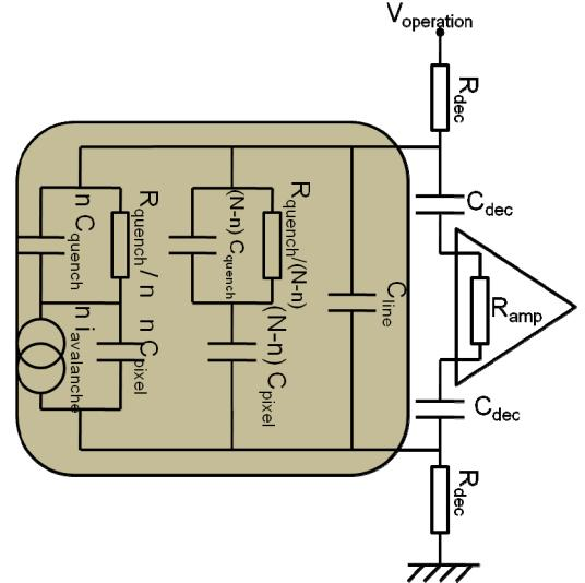
Fig. 1. Schematic of a MPPC and associated electronics. The MPPC is enclosed in the brown box. The model is inspired from [4].
