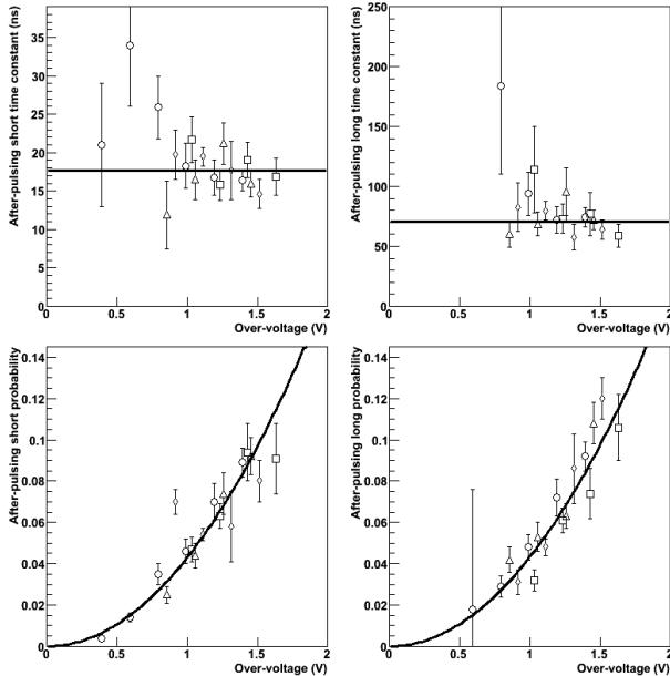
Fig. 4. After-pulse measurement. Each symbol represents a different MPPC. The average time constants are 17 and 70ns. The probabilities follow roughly the same dependence  $0.04 \times \Delta V^2$ .
