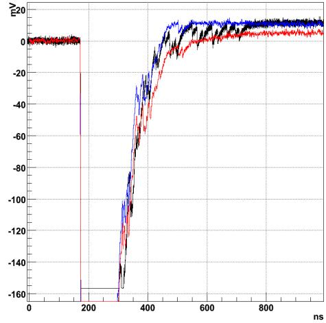
Fig. 6. Comparison of waveform for data (black) and simulations (blue and red). Two different pulse shape were used for the simulated waveforms: SPICE for the blue, empirical for the red.
