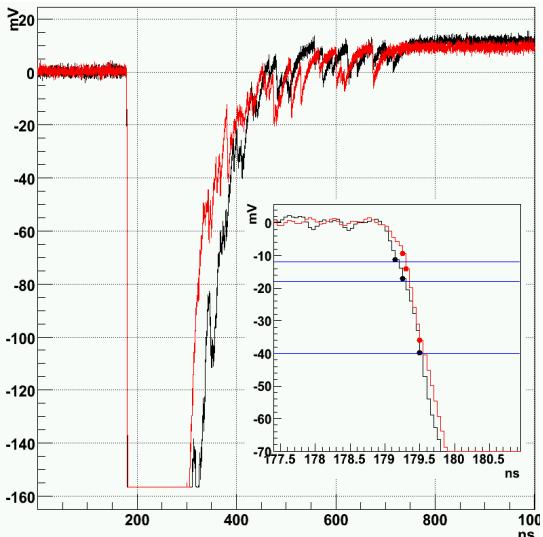
Fig. 3. Typical waveform recorded when both pulse height fall within the 511 keV window. The inset shows a zoom along the rising edge of the pulse. The lines show the location of the thresholds used to estimate the time, -40 mV, -18 mV and -12 mV from bottom to top.
