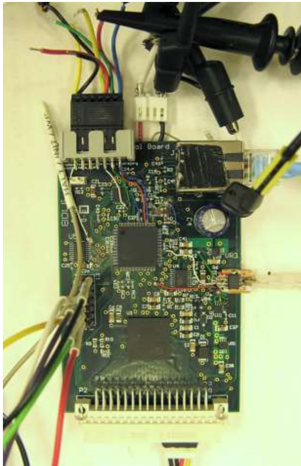
Figure 43: Photograph of one of the digital control boards during testing, including the diagnostic signal output header at the top left
