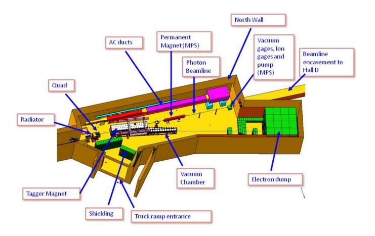
Figure 2 Layout of the major equipment in tagger hall showing the location of the tagger magnet and vacuum chamber.
