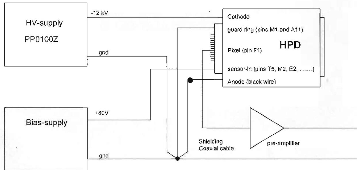
Bias voltage connections: pins T5, M2, E2, A5, A12, E15, M15 and T12
