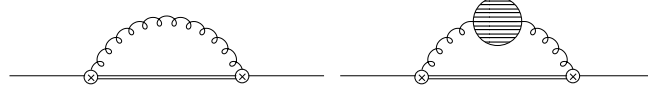
Figure 1: The diagrams contributing to our calculation. Single lines are colour-singlet Q\bar{Q} states, double lines are colour octets, curly lines are gluons, vertices are chromoelectric dipoles and the blob is the gluon self-energy. The imaginary part of the first diagram yields the singlet-to-octet decay mechanism, whereas the second one gives the Landau damping contribution to the width.
