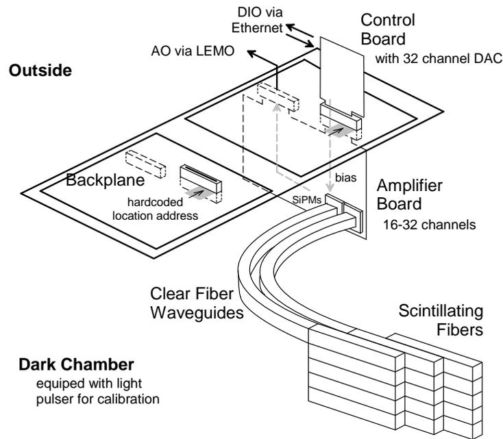
Figure 5.1: Diagram of the readout scheme of the tagger microscope. The SiPMs are connected to the scintillating fibers through clear fibers so that they can be mounted out of the radiation zone near the mid-plane of the spectrometer.
