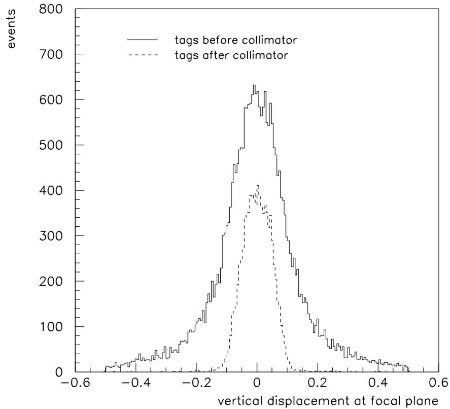
Figure 5.2: The distribution in vertical coordinate of the post-bremsstrahlung electrons at the tagger focal plane in the region of the coherent peak, for all tags (upper curve) and those that pass the photon collimator (lower curve). When all fibers except the central row in the microscope are inhibited, only electrons with  $|y| < 1$  mm contribute to the tagging rate.
