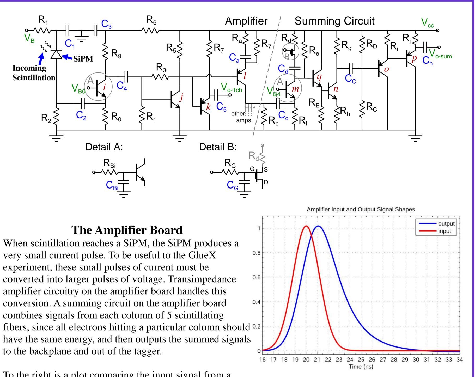
To the right is a plot comparing the input signal from a SiPM to the output signal from the amplifier. The signal amplitudes have been normalized for easier comparison of the signal shape. The plot shows that the amplifier responds within 1 ns, and creates a pulse that rises with a shape very similar to shape of the SiPM signal.
