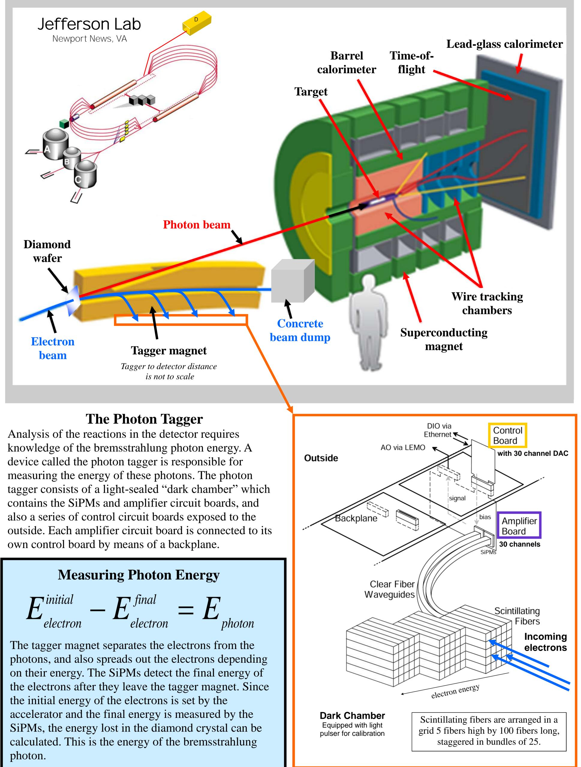
Analysis of the reactions in the detector requires knowledge of the bremsstrahlung photon energy. A device called the photon tagger is responsible for measuring the energy of these photons. The photon contains the SiPMs and amplifier circuit boards, and also a series of control circuit boards exposed to the own control board by means of a backplane.
