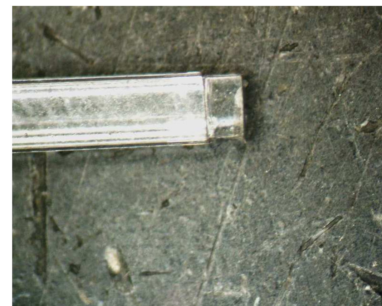
Figure 3: The first step: trimming back the cladding and exposing the core.
