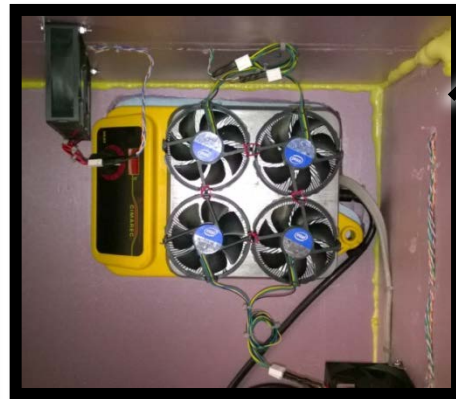
Hot plate with thermally bonded heat sinks/fans
