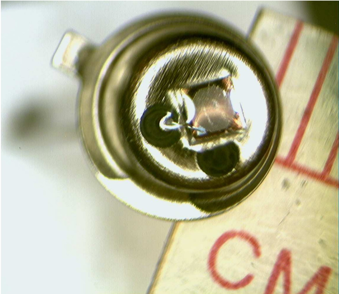
Figure 3: Photonic device SSPM-050701GR-TO18: 1 \times 1\text{mm}^2 sensitive area with 556 pixels. Note the millimeter markings for scale.
