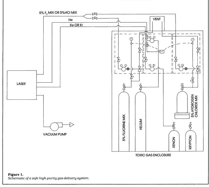
exhaust flow to prevent diffusion of any leaked gas back into the room. A vented cabinet should be designed to allow the user to close a cylinder valve without allowing any gas to enter the room.
