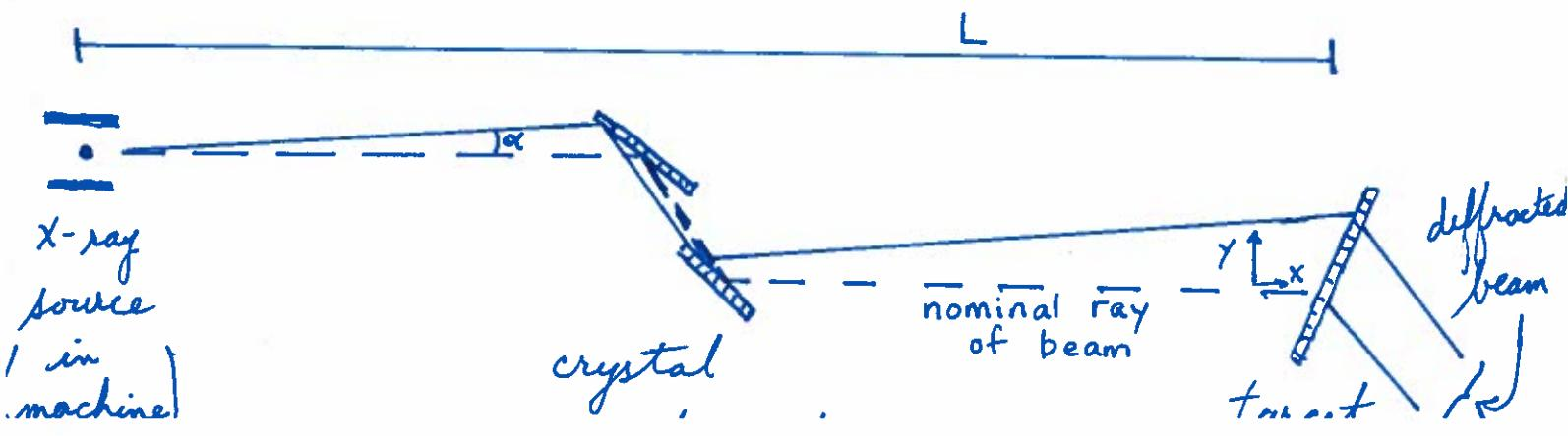
The nominal ray indicated by the dashed line is presumably the center of the beam, and all other rays accepted by the beam slits are indicated by values of  $\alpha \neq 0$ . At the position of the target, a ray of angle  $\alpha$  strikes the target at height  $y$  from the beam axis, where
