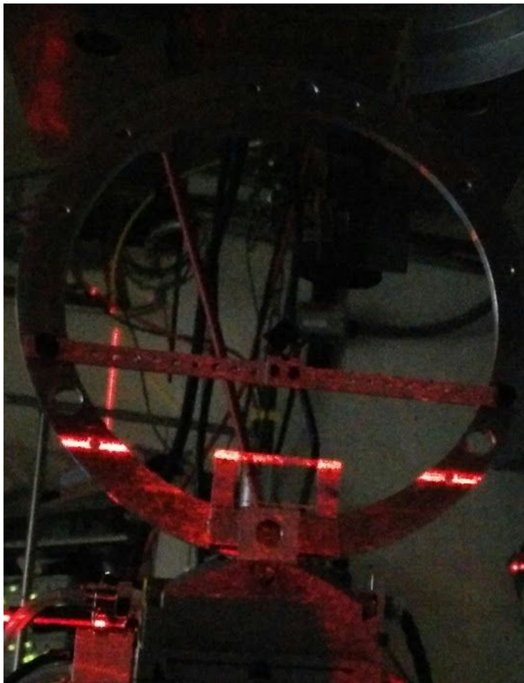
Picture of the horizontal chi reference. Notice the red laser is centered on the two bolt holes. The chi angle when this occurs (with theta = 0) becomes the reference against which crystal chi offsets are measured.
