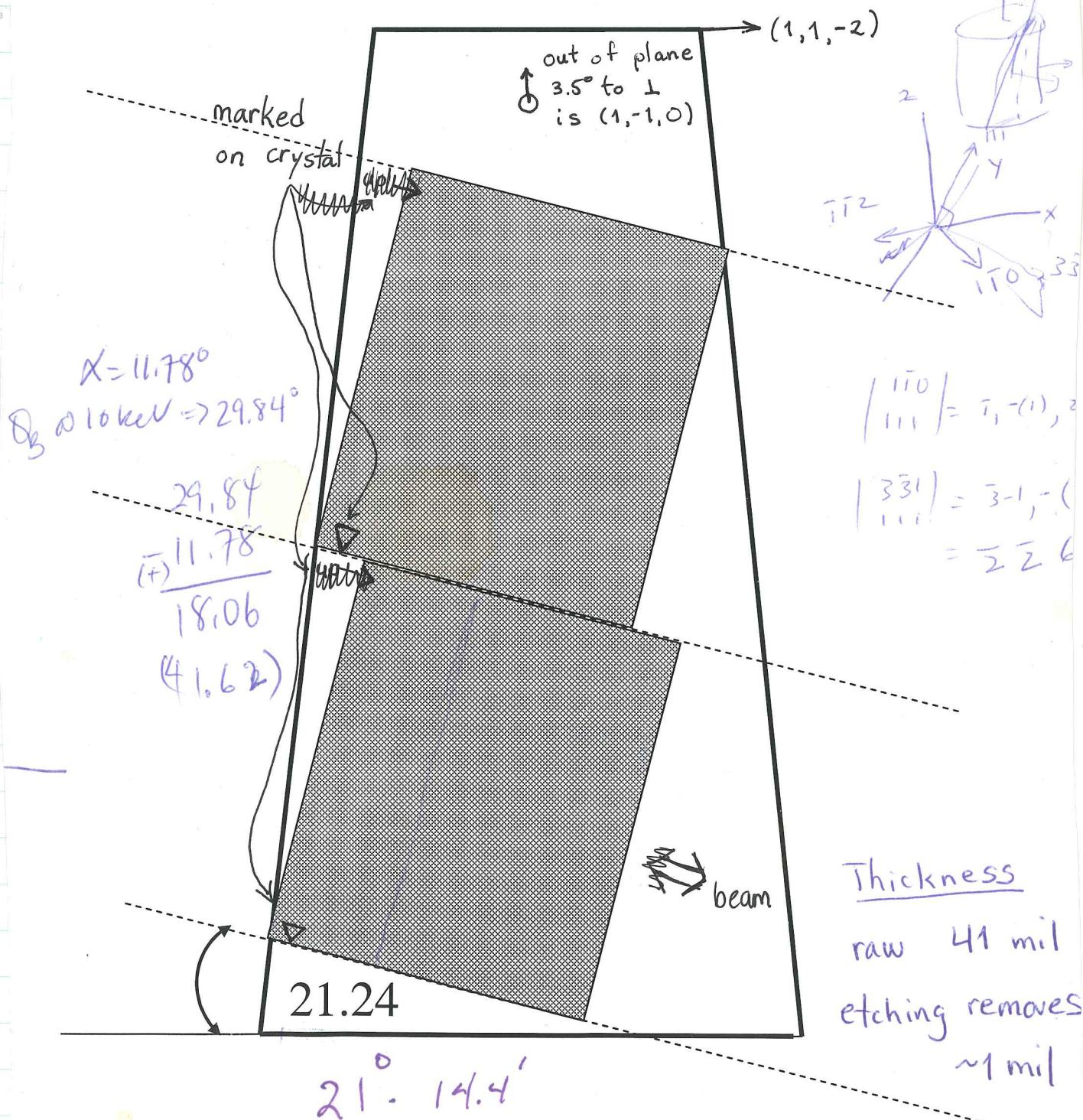
The original wedge was cut from a 111 silicon ingot as shown below. The ingot is a cylinder with one flat side.
