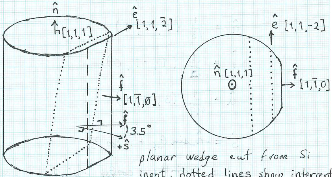
planar wedge cut from Si ingot; dotted lines show intercepts with the boundaries of the ingot
