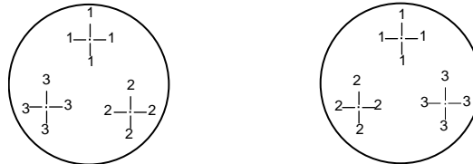
Fiducials assigned to two data arrays in which numerical order is not followed. This will produce a significant out-of-tolerance error.
