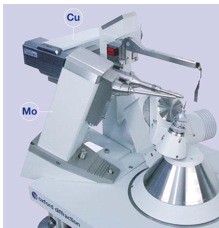
Co-mounted Enhance Ultra (Cu) and Enhance (Mo) X-ray sources
