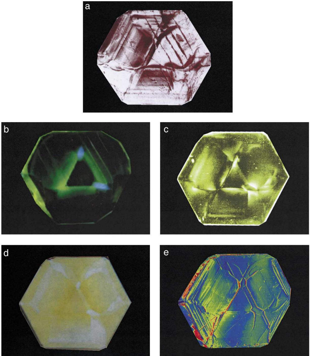
Fig. 1. Results of diamond characterisation, size:  $10 \times 12 \text{ mm}^2$ . (a) X-ray white beam topograph of an as-cleaved diamond crystal. (b) XEOL picture of a sample adjacent to the one shown in (a). (c) Polarised light optical micrograph of the sample thinned down to 0.42 mm. (d) Close-up photograph. (e) Rocking curve FWHM contour maps of the thinned diamond recorded with the FReLoN camera; colours (mdeg): blue: 1.25, green: 1.5, yellow: 1.75, orange: 2, red: 2.25.
