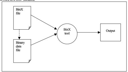
Figure 1. Showing how the BinX file is used in to describe the format of the binary file.
