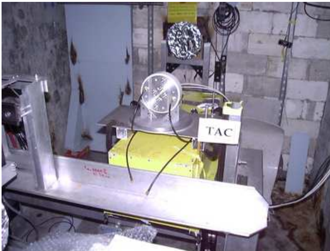
FIG. 1: Photograph of the prototype active collimator installed on top of the total absorption counter in Hall B, as configured for the parasitic beam tests in April 2007. The detector was mounted so that its central hole is at the height of the electron beam while the TAC is in its parked position below the lead brick wall that shields it from the direct photon beam. It was then horizontally scanned across the beam by moving the TAC left and right.
