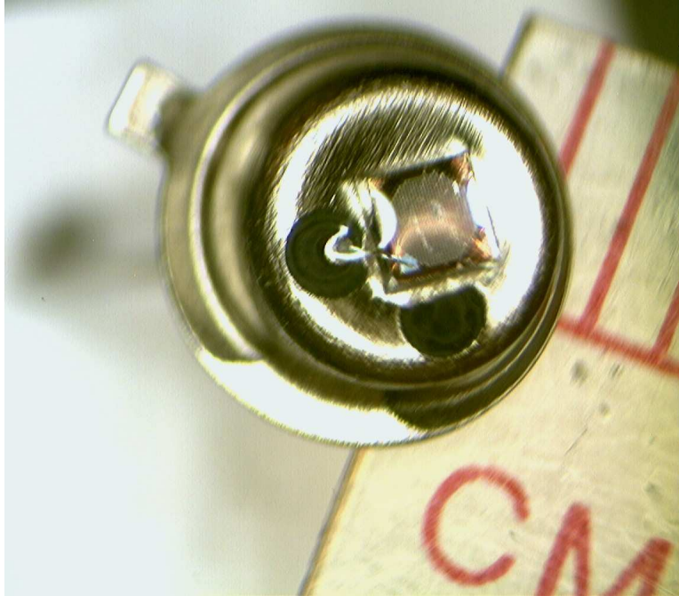
Figure 1: Photonique device SSPM-050701GR-TO18: 1 \times 1 \text{ mm}^2 sensitive area with 556 pixels. Note the millimeter markings for scale.
