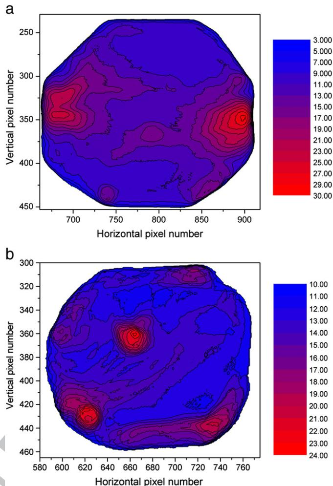
Fig. 1. Maps of rocking curve width for the (2,2,0) planes of two diamond crystals, taken under diffraction conditions described in the text. Each pixel subtends a region on the diamond that is 23  $\mu\text{m}$  (horizontal)  $\times$  24  $\mu\text{m}$  (vertical). (For interpretation of the references to colour in this figure legend, the reader is referred to the web version of this article.)
