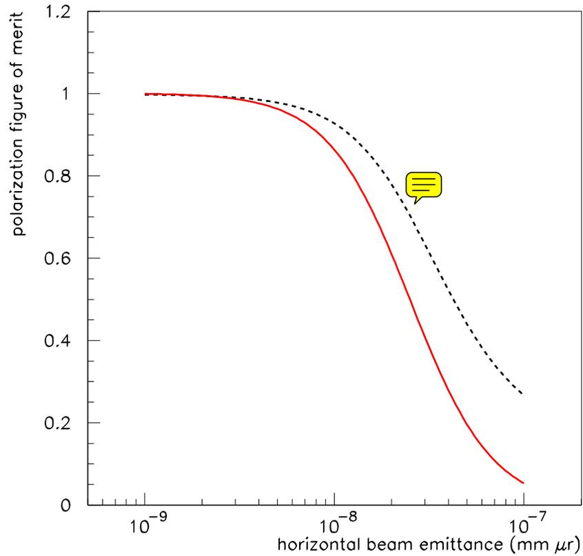
Figure 3: Polarization figure of merit as a function of horizontal electron beam emittance, under nominal conditions for the Hall D photon beam collimator, assuming that the operating current is determined by the background rate (dashed curve) or tagging accidentals rate (solid curve). The electron beam energy is 12 GeV. The primary coherent peak is at 9 GeV, with the tagger set to tag photons between 8.4 and 9 GeV.
