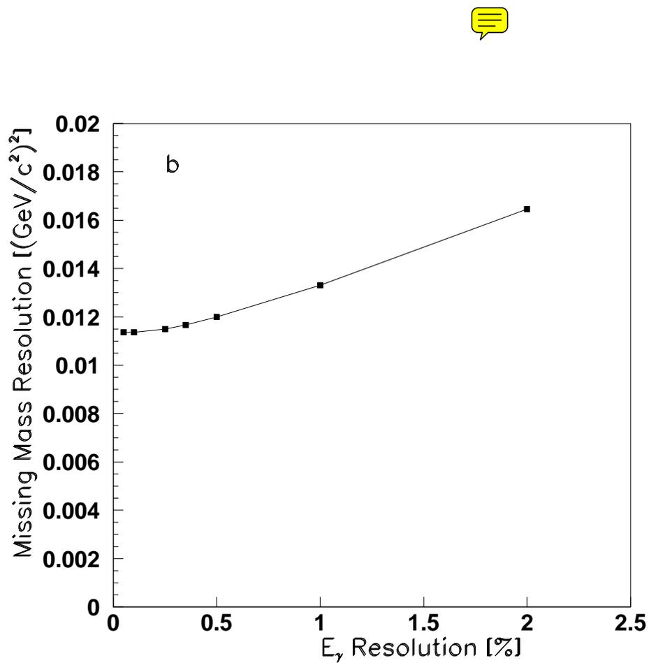
Figure 4: Missing mass resolution as a function of the uncertainty on the initial state photon energy measured by the tagger. The reaction used for this study was  $\gamma p \rightarrow K^+ K^- \pi^+ \pi^- \pi^0 p$  where the  $\pi^0$  is undetected and must be reconstructed using missing momentum. The incident photon energy is 9 GeV.
