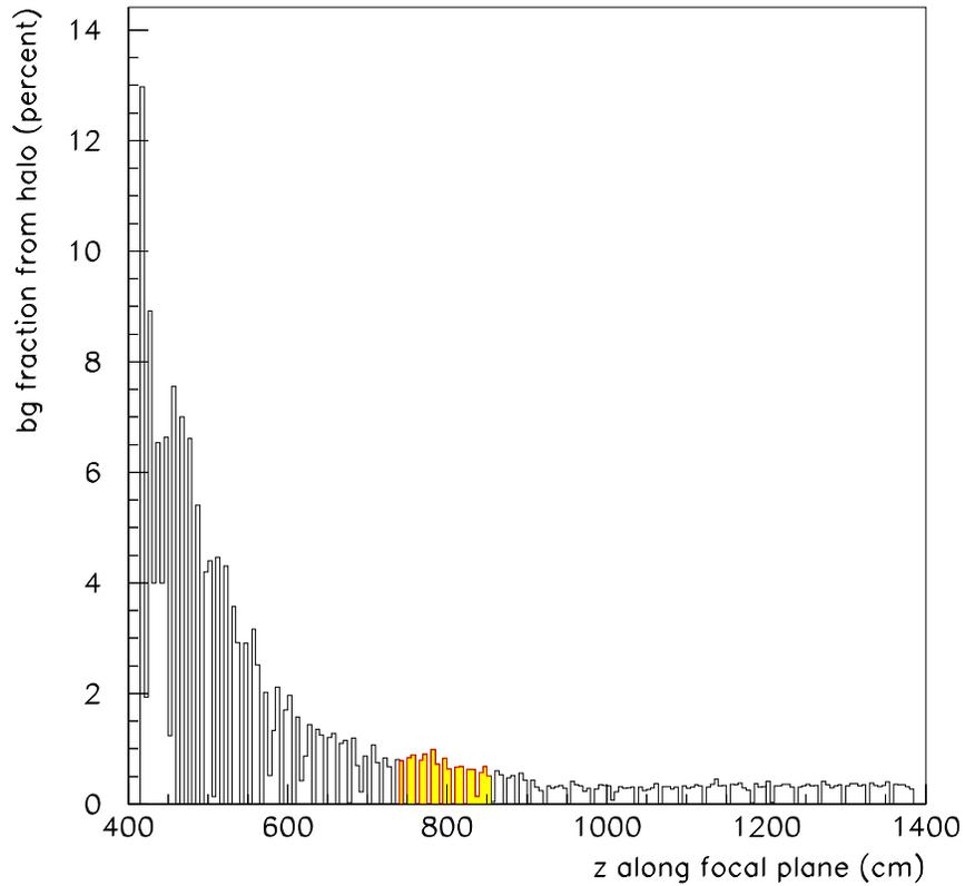
Figure 6: Percentage of hits in the broad-band tagging counters that are generated from electron beam halo particles, assuming a beam halo fraction of  $10^{-5}$ . The electron beam energy scale is roughly linear in the  $z$  coordinate, varying from 600 MeV at the left end of the plot to 9 GeV at the right. The shaded region indicates the coverage of the microscope.
