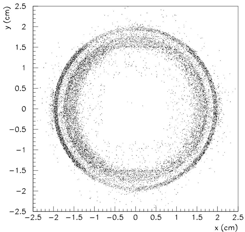
Figure 5: Transverse profile at the radiator of particles in the beam halo that went on to create hits in the tagger focal plane counters. Each point is the intersection of an electron track with the plane containing the radiator. The crystal radiator is in the center of the frame, but is invisible in this image because it is so thin that relatively few electrons interact in it.
