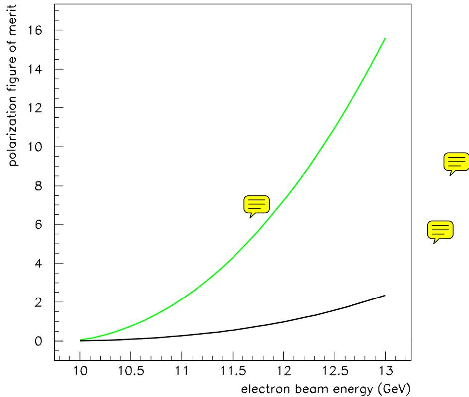
Figure 1: Polarization figure of merit (arb. units) as a function of electron beam energy with (upper curve) and without (lower curve) photon beam collimation. The collimator is the nominal 3.5 mm diameter circular aperture located 75 m downstream from the radiator. An electron beam emittance of  $10 \text{ mm}\cdot\mu\text{r}$  is assumed.
