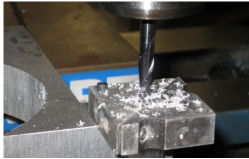
FIGURE 10. The light guides are being milled to specified length. The fiber debris must be cleared before the next pass of the end mill over the fiber end surface.
