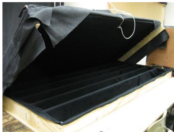
FIGURE 11. A photo of the intermediate storage box for the fibers in production.
