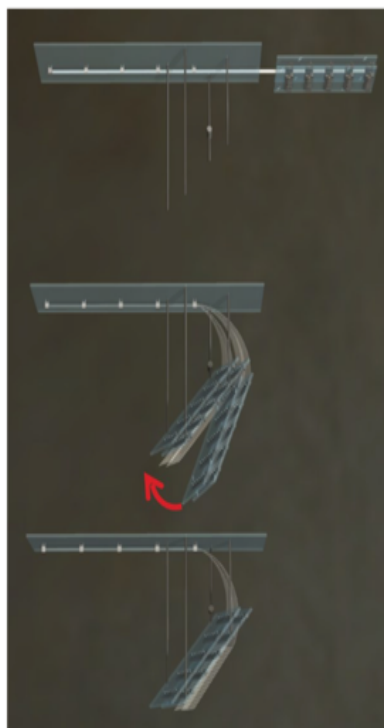
FIGURE 26. A rendering of the chimney plates being secured to the bending plate.
